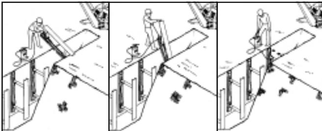
Set-up and position shore at edge of trench, and connect pump hose
