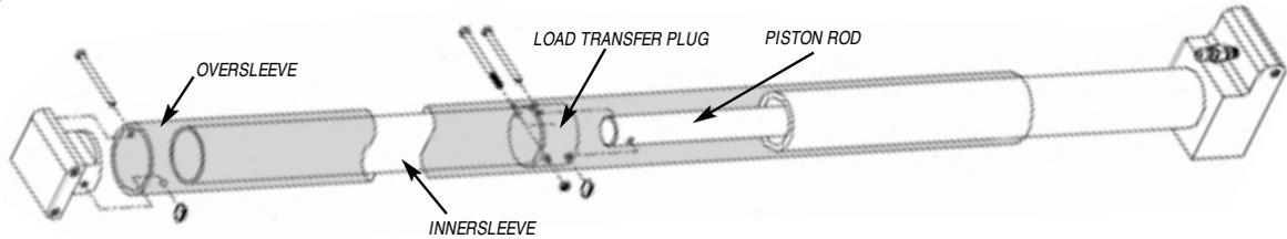
Cylinder extensions are a convenient and efficient means of extending the minimum and maximum working range of shores. Reusable, lightweight aluminum extension units are easily connected to each cylinder in the field. Such versatility allows shoring of various trench widths with the same shores. Cylinder extension units are pre-assembled for ease of attachment, and include all connecting hardware.
