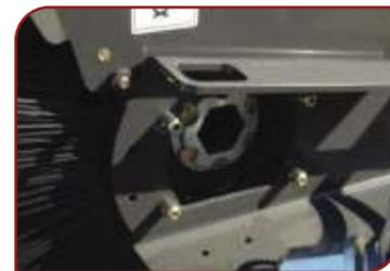
Pull out the motor and hex drive assembly. The core/brush head will fall out. Hydraulic hoses do not need to be removed.
