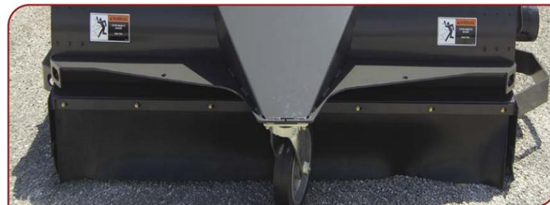
A double drape system seals the sweeping chamber to the ground
