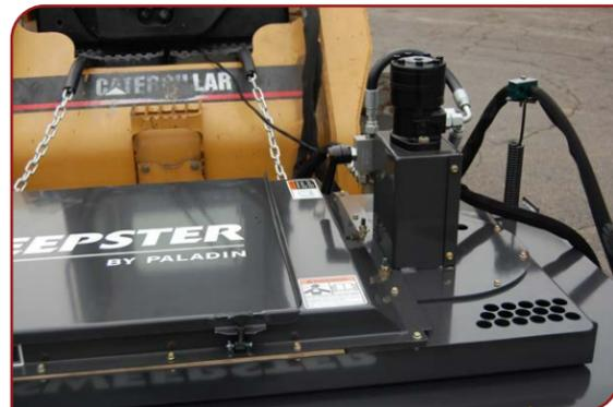
High volume hydraulic fan pulls air from the sweeping chamber filtering the dust and exhausting clean air
