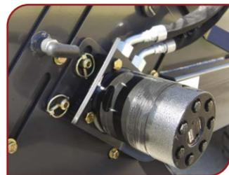
After resting the sweeper on the ground, remove the pins from motor and bearing mounts
