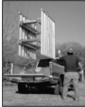
Lightweight aluminum construction allows for transport in light-duty trucks. Systems may be transported fully assembled, or in "component form" when space is limited.
