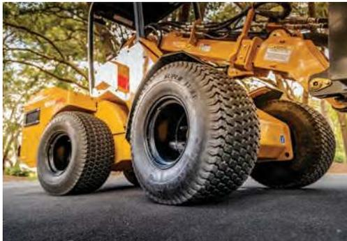
Equipped with turf tires provides a light footprint and minimal turf interruption.
