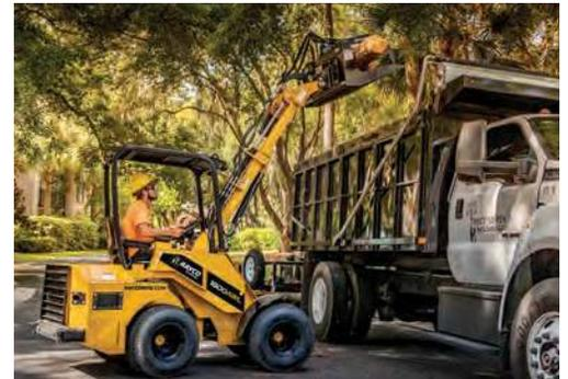
Standard telescoping boom provides excellent dumping and lifting height.
