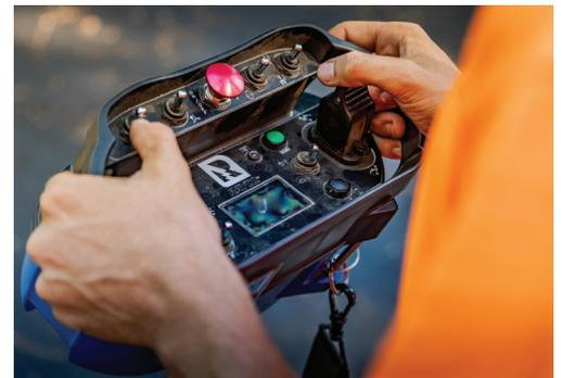
*The wireless remote control unit is comfortable and sealed against dust, water, and other elements.*
