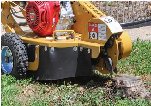
Equipped with Rayco Super Teeth<sup>®</sup>: forged, one-piece design with tungsten carbide tips.
