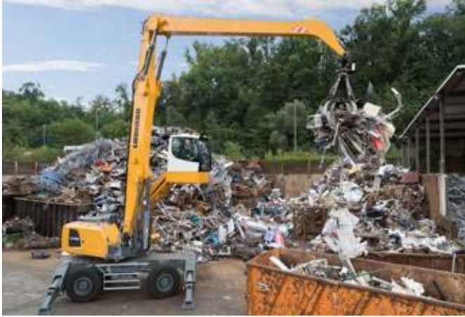
LH 50 M Industry Litronic in scrap handling operation
