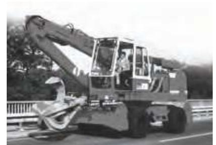
First hydraulic cab elevation
