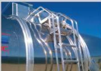
Double Top Step Ladder with Safety Handrails
