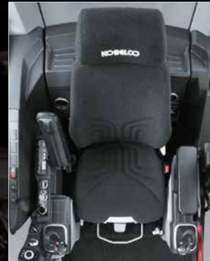
GRAMMER air suspension seat is standard. It has superior shock absorption and can be used for long periods of time and reducing fatigue.
