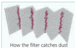
\* "60-mesh" means that there are 60 holes formed by horizontal and vertical wires in every square inch of filter.
