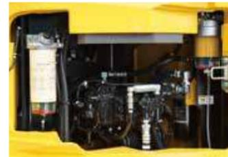
Fuel filter with built-in water-separator
