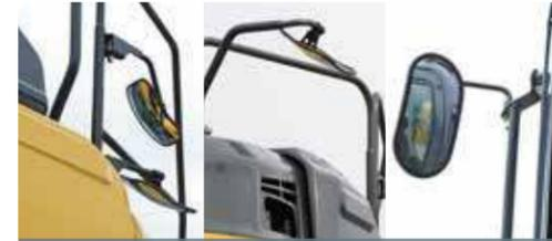
Left and right rear-view mirrors / Right bottom clearance mirror
