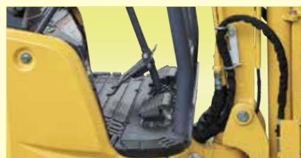
Pass-through operating station allows getting on and off from either side.
