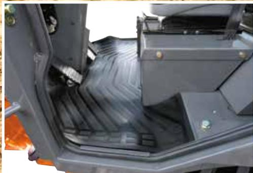
The flat cab floor enables easy cleaning.
