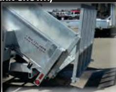
**Double-Acting Spreader End Gate (STD on DT & DT-DO)**
