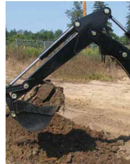
Several classes available depending on desired weight & digging force. 180° bucket rotation and swing arc. Heavy-duty construction grade available for heavy-duty applications. Equipped with cushioned cylinders.
