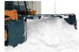
Efficiently moves large volumes of snow. Ideal for waste water, manure, feed lots, and flow clean-up. Optional pull back kit draws snow from buildings, fences and confined areas. Cutting edge trip system allows operator to glide over manholes and curbs without losing gathered materials.
