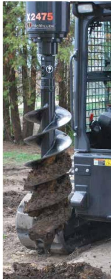
75 Series drive units are completely sealed with all moving components running in oil for total lubrication on a constant basis. The 75 Series hydraulic motor drives the auger through a sealed planetary gear reduction.
