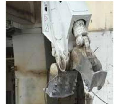
UPX 950 WITH CONCRETE PULVERIZER JAWS
