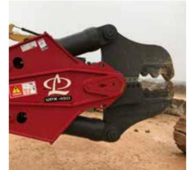
UPX 450 WITH CONCRETE CRACKING JAWS
