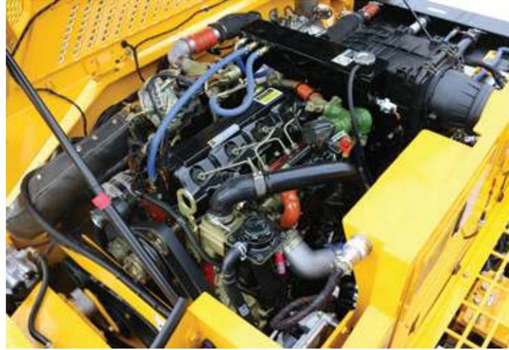
*The layout of the engine, hydraulics and electrical, along with its forward-tilting hood and large side doors, make service and maintenance easy and accessible.*
