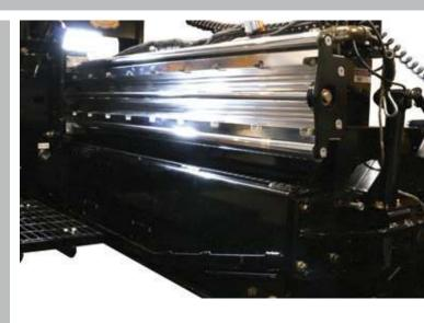
Featuring fully adjustable slide block bushings and an extruded aluminum slide track frame the EZV delivers class-leading extension support and integrity for reduced component lifecycle costs and superior performance.
