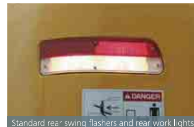
Standard rear swing flashers and rear work lights.
