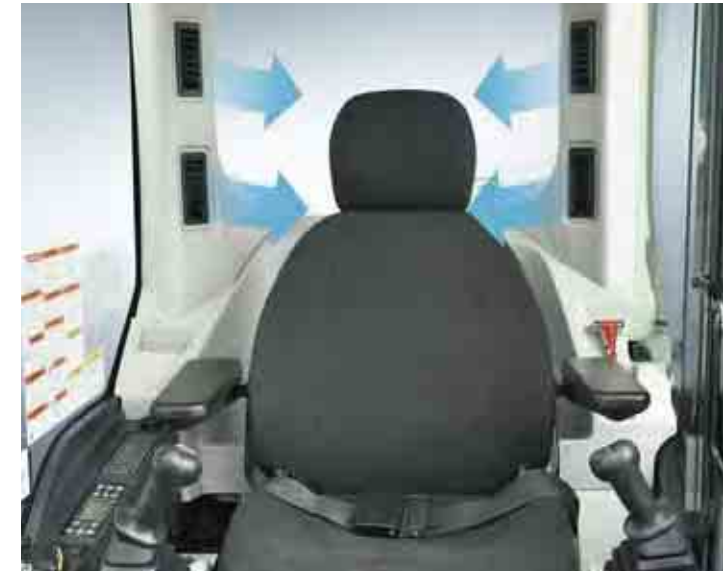
Five air outlets deliver warm or cool air directly to the operator.
